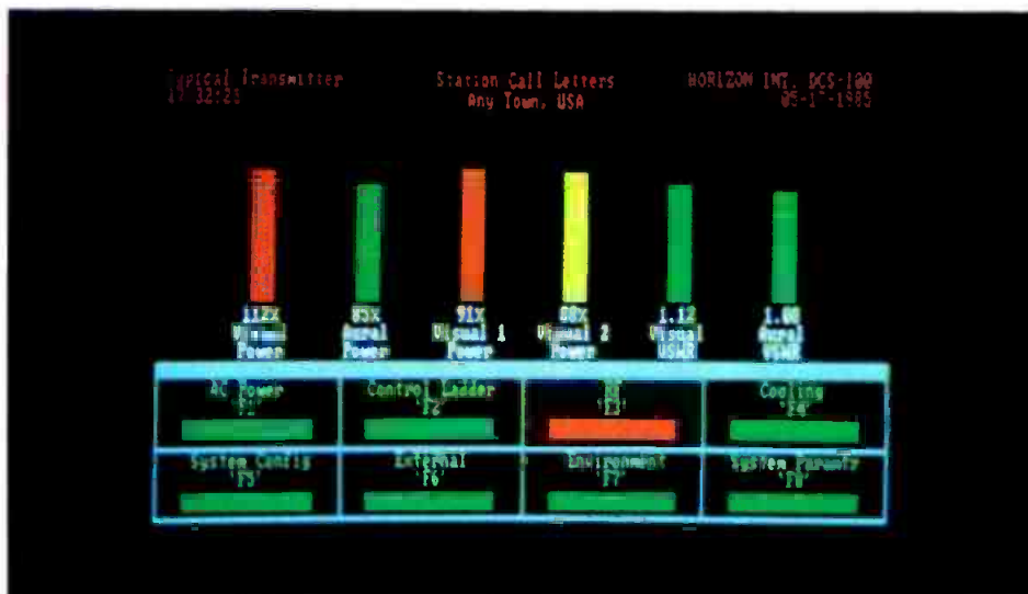
Figure 2. Bar-graph display with transmitter parameters out of tolerance. Red represents power out of range. Yellow represents a cautionary condition.
